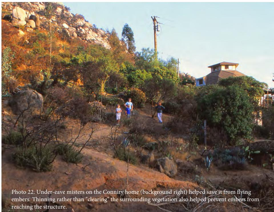
Photo 22. Under-eave misters on the Conniry home (background right) helped save it from flying embers. Thinning rather than "clearing" the surrounding vegetation also helped prevent embers from reaching the structure.
