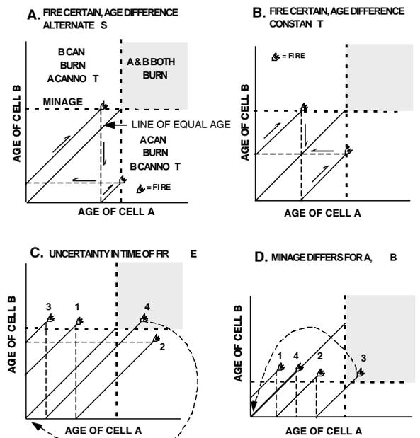
initial condition  $a_A \neq a_B$ . Thus the boundary between the two cells is an age boundary. MINAGE, following the definition above, is the minimum age at which a fire can be carried. We also assume that each cell has a probability  $p$  of being burned in each year. If a fire occurs, and the age is equal to or greater than MINAGE, the cell burns. If the age of the other cell is less than MINAGE, it cannot burn. If it is greater than MINAGE fire will spread into it and both cells will burn.
