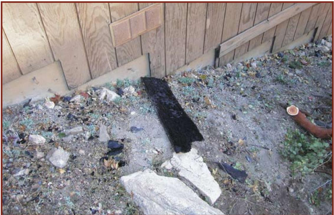
Post-fire visual examination indicated a lack of substantial fire effects on the vegetation and surface fuels between burned homes. Lack of surface fire evidence in surrounding vegetation provides strong evidence that house-to-house ignitions by airborne firebrands were responsible for many of the
